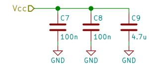
Place decoupling capacitors as close to power inputs on microcontroller as possible.
