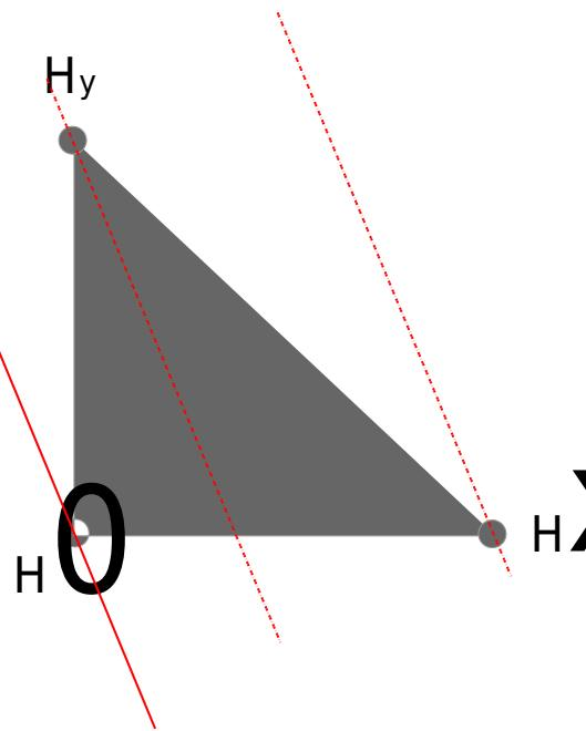
Because the wave emanating from the pinger hit  $H_x$  before it hit  $H_0$ , we know that  $H_x$  must be closer to the pinger than  $H_0$ . In fact,  $H_x$  must be exactly  $d_x = c_s(t_0 - t_x)$  meters closer to the pinger than  $H_0$ . Likewise,  $H_y$  is  $d_y = c_s(t_0 - t_y)$  meters closer to the pinger
