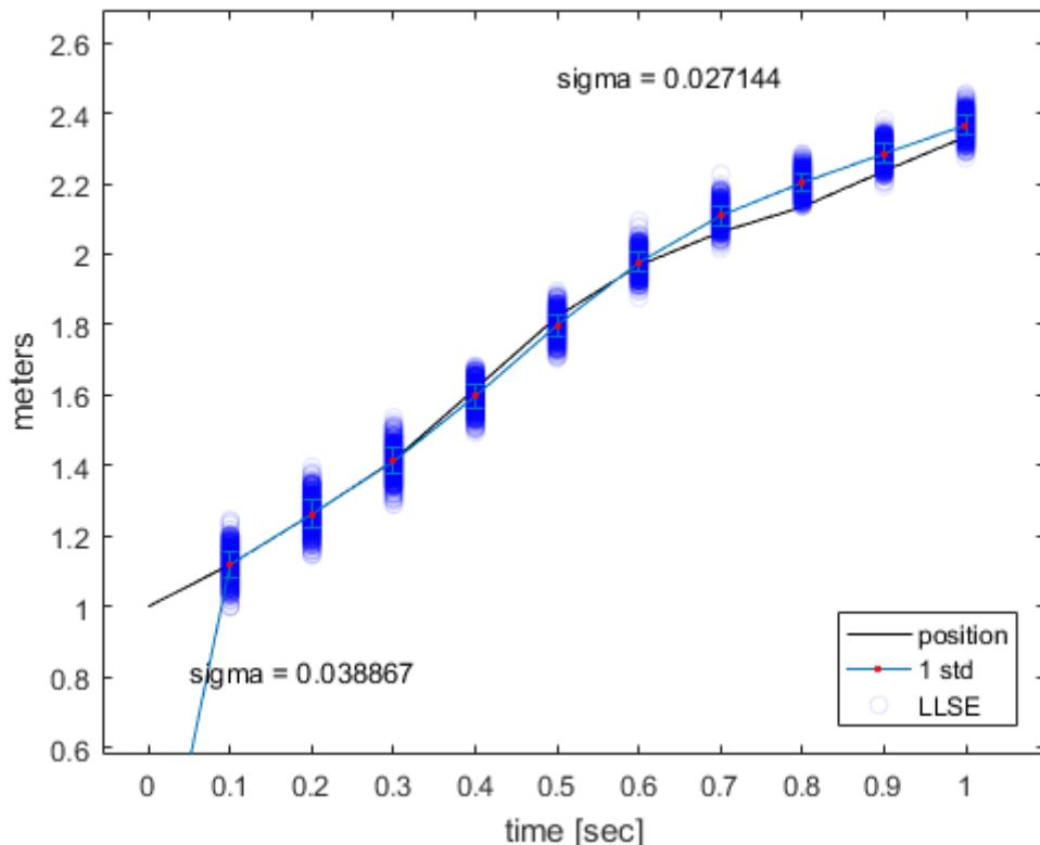
Notice how originally, the std of the estimation is close to \$0.04m\$. That's exactly what we'd expect from just using 4 depth sensors with  $\sigma = 0.08m$ . However as time goes on and more estimates are made, the noise of the position estimate drops to around \$0.027m\$.
