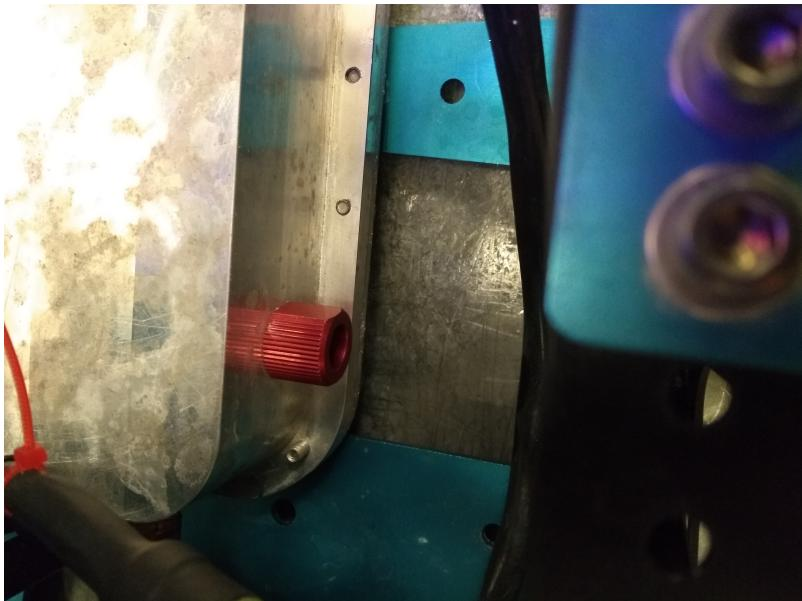
2. Plug the sensing cable into the SeaCon connector on the battery box.
