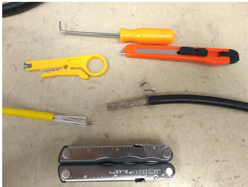
Remove the outer jackets of both cables
