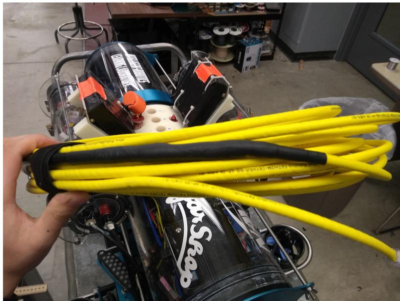
Slide the large heat shrink over the splice and shrink it down with the heat gun at 90 degrees Celsius. Make sure it is completely shrunk down and you're done!
