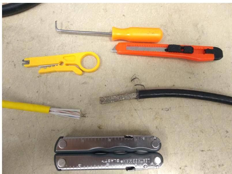
Remove the outer jackets of both cables
