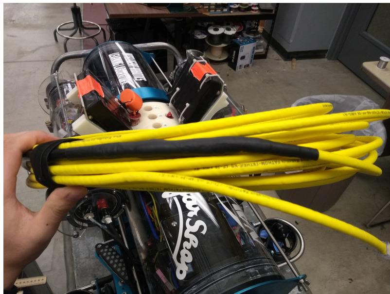
Slide the large heat shrink over the splice and shrink it down with the heat gun at 90 degrees Celsius. Make sure it is completely shrunk down and your done!
