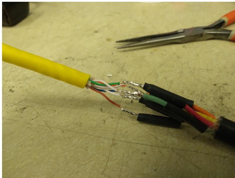
Solder the wires together. Make sure the heat shrink doesn't shrink too much in this stage from the soldering iron. Too much will render the heat shrink unusable.
