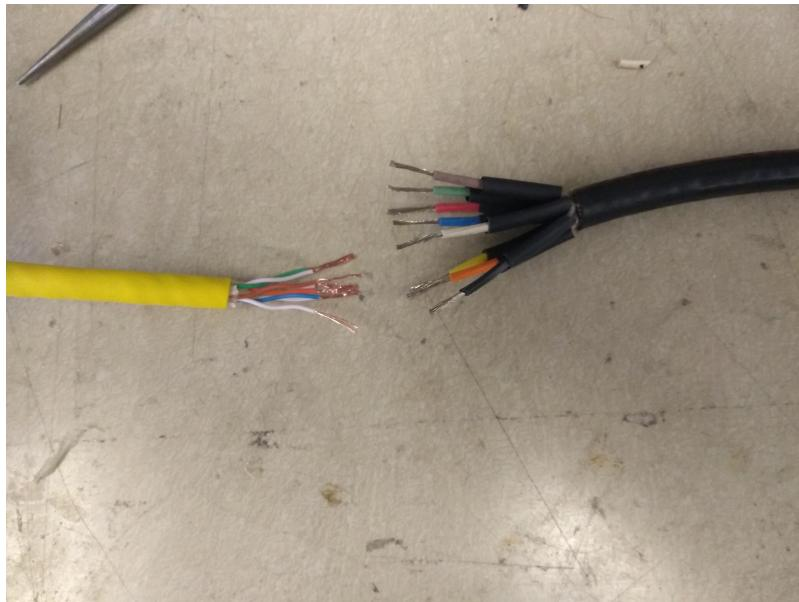
Make sure there is enough bare metal that there is enough length for each bare wire to wrap around each other. Also make sure the small heat shrink is long enough to cover the solder joint.
