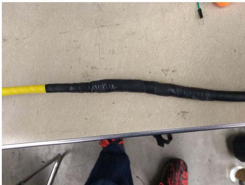
Wrap the splice in electrical tape. Start with a few wraps on one side, have the tape overlap half of itself as it winds up the splice and then end with a few wraps on the opposite side. Make sure the heat shrink is tight.
