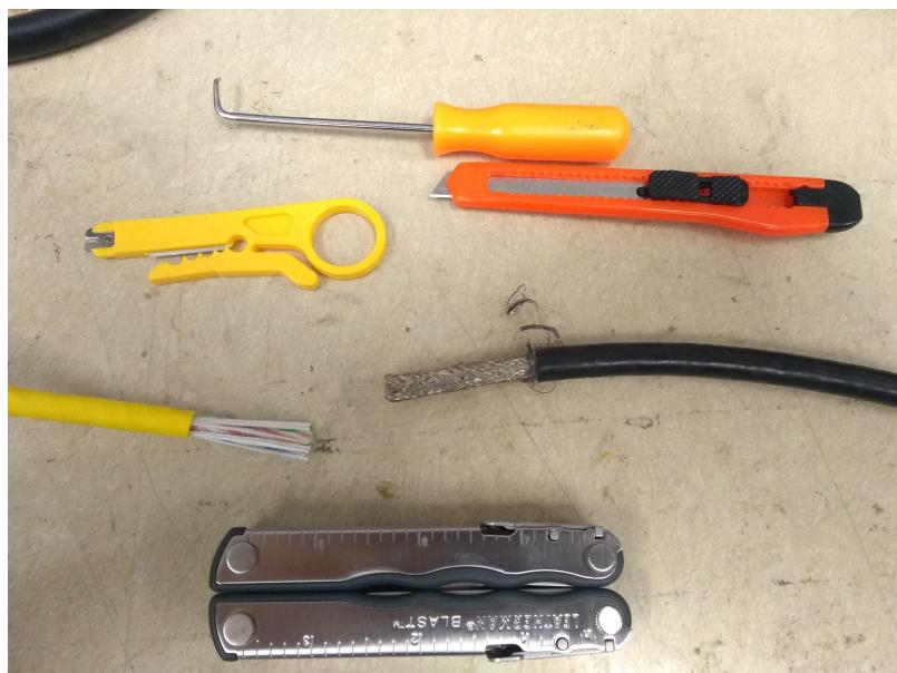
Remove the outer jackets of both cables
