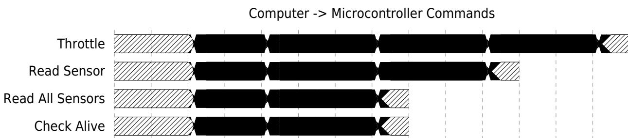
The first two commands are the basic interface for controlling the thrusters and getting information. There is the third macro command for reading all the registers of a thruster. There is no macro command for talking to all thrusters because this would require the microcontroller to know what thrusters exist/are active on the sub, which would complicate the code. The final command is a method for checking if a thruster is alive and responding, it will return a bool true/false value.
